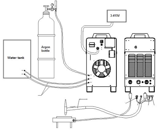
6.1 The power supply of this machine is 3~380V 50/60HZ, user should prepare the switchboard and install the air switch (breaker) and ground cable. Connect the green-yellow wire of the three-phase input cable to the grounding wire on the switchboard reliably according to the below table:
